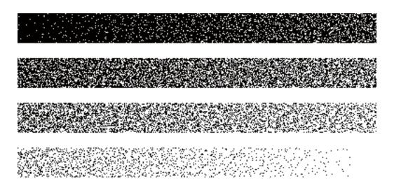
Figure 2(b). Gray Scale Ramp by Random dot pattern method
